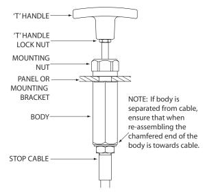
6. Valves fitted with the manual shut down handle assembly RTD-100. Fit through a suitable Ø20mm (3/4") hole in a bulkhead or mounting bracket as follows. Release the handle locknut. Remove the handle, handle locknut and upper locknut and washer. Thread handle body through the bulkhead/bracket. Refit upper locknut and washer. Adjust lower and upper locknuts to position handle and tighten. Refit handle locknut and handle. Tighten locknut.
